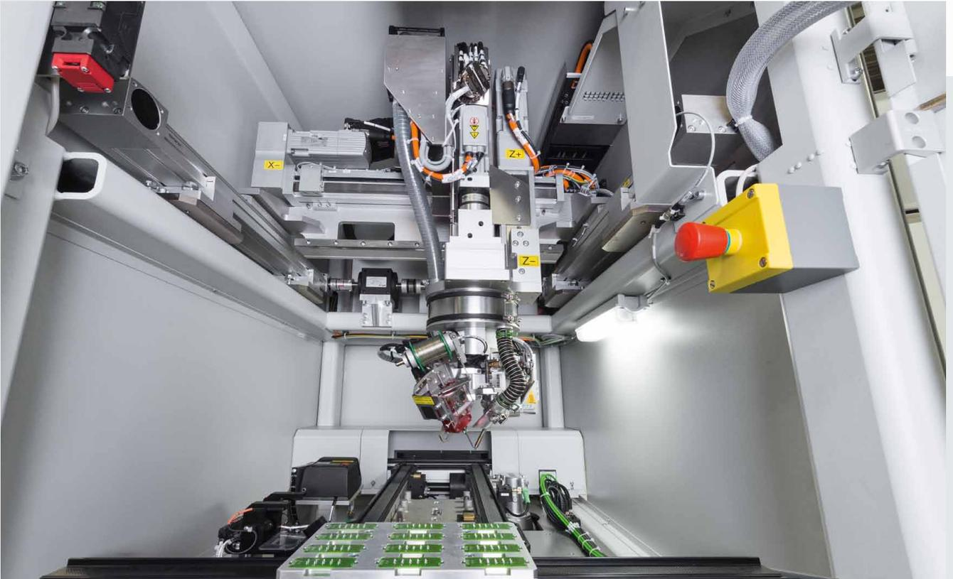
**Reliable handling, reliable operation:** spindle axis EGC, toothed belt axis EGC with integrated displacement encoder, electric slide EGSL plus a customised module based on the ERMB.
