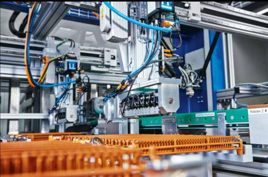
**The electric axis EGC-HD, known for its rigidity and precision, moves a mechanical gripper horizontally. This lifts several parts at a time, swivels 90° and sets them down in a lattice tray.**
