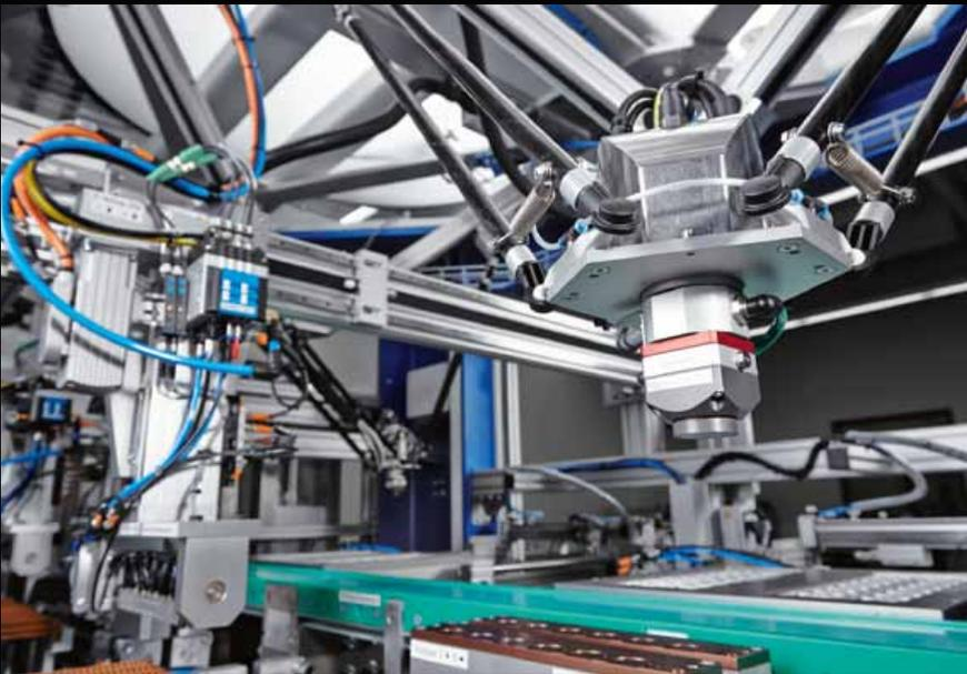
**The delta robot uses a specially developed vacuum gripper to pick up the parts from the conveyor belt and set these down in either a lattice tray or JEDEC tray.**
