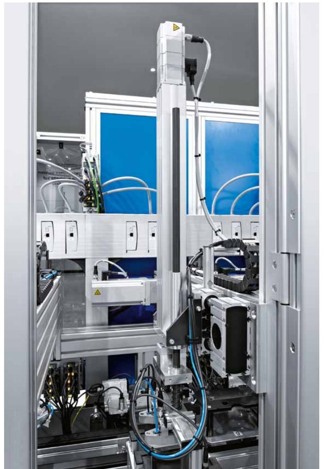
**Storing bipolar plates** In this handling system, the stepper motors of electric cylinder EPCO and toothed belt axis ELGR are actuated by servo controller CMMO-ST.
