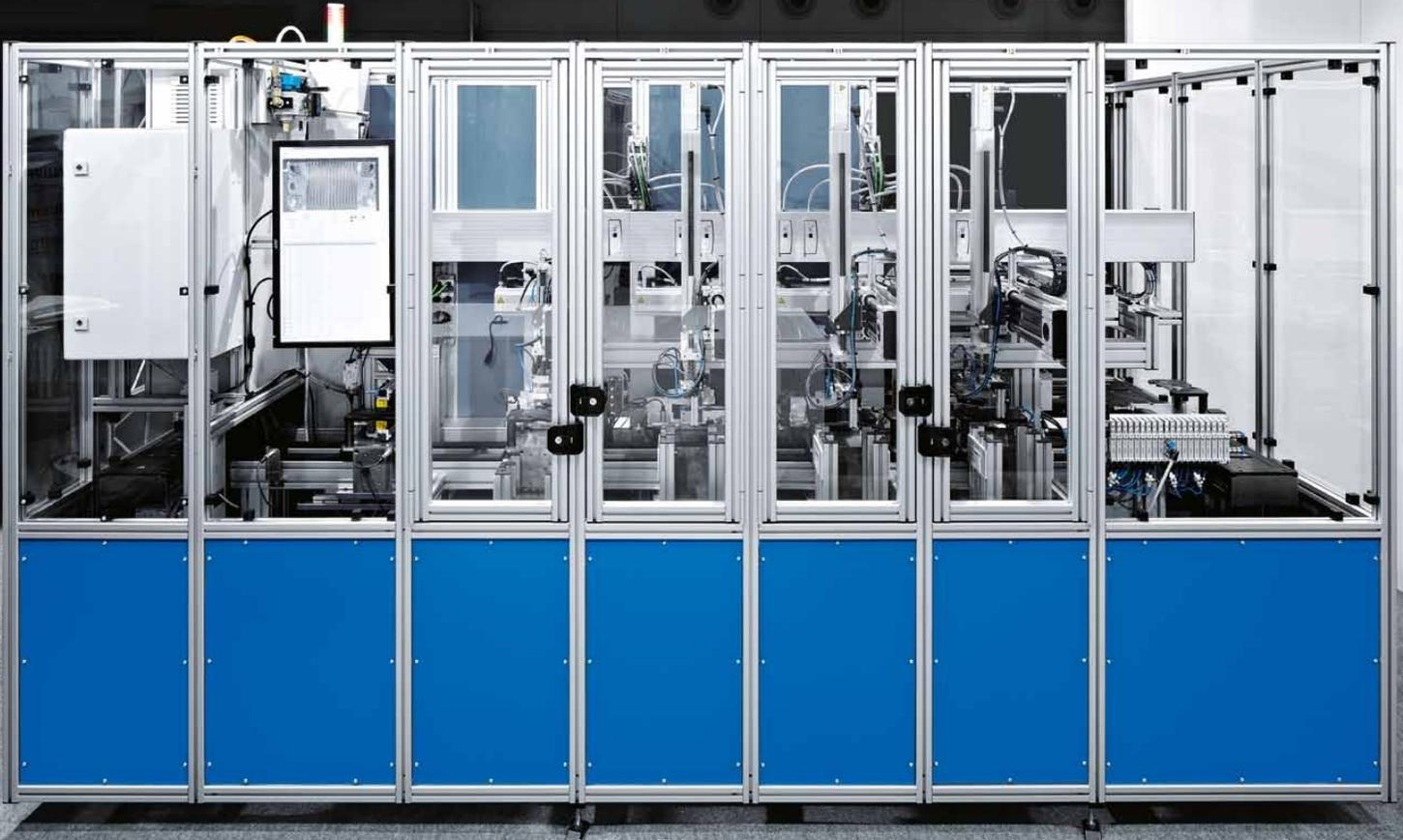
Quality for high efficiency: The new system from P+K checks the thickness and surface finish of bipolar plates.
