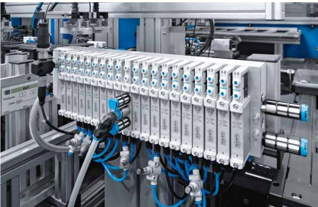
**A valve terminal VTUG**, connected to the master controller via IO-Link, controls all the pneumatic actuators in the system.
