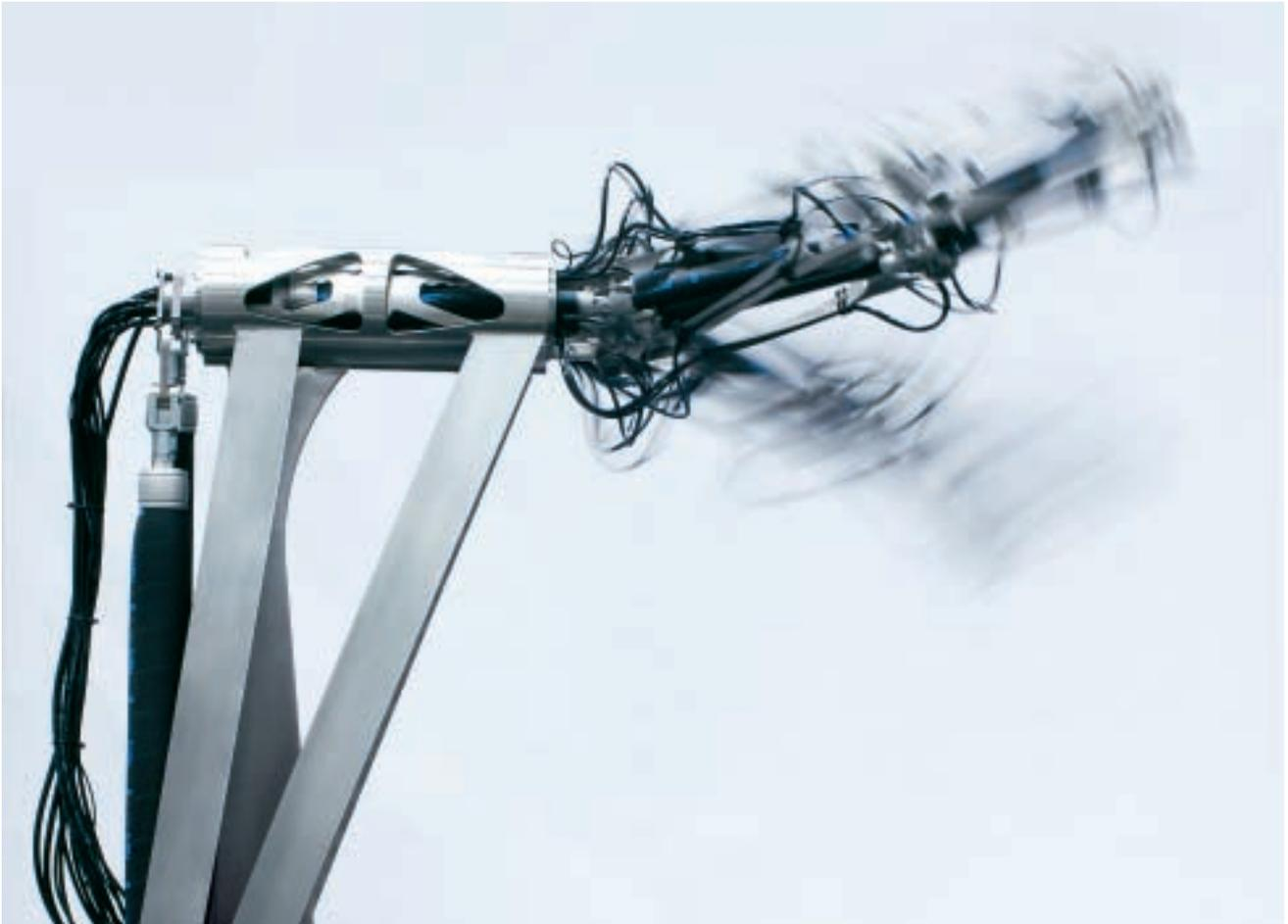
Biologically inspired by analyses of lobsters' and grasshoppers' legs and of human pointing gestures, a two-segmented arm with an external skeleton has been developed with movement patterns similar to those of a human. Powered by pneumatic muscles, "AirArm" catches drops of water.
