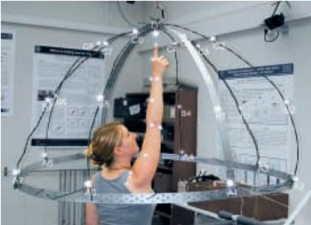
Experimental setup. Arm and target of the reaching movement are marked by reflective balls.
