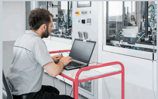
Fig. 2: Commissioning an axis system using configuration software → Festo Configuration Tool (FCT)
