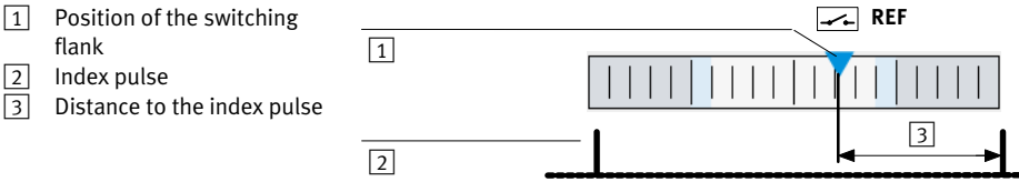
Fig. 2.3 Alignment of the reference switch during index evaluation
