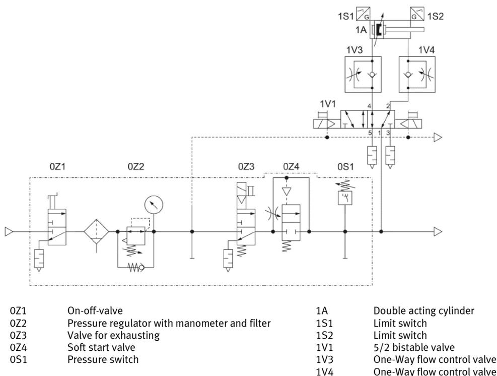
Figure 4 Standard circuit with service unit for depressurisation of the system with the additional function of switching the power valves to any position
