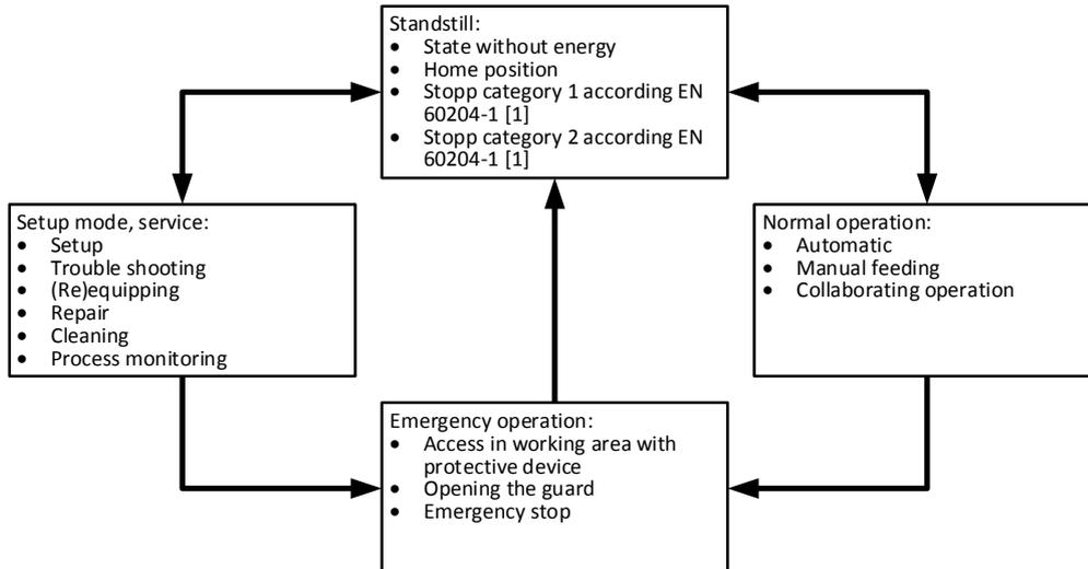
Figure 2: Sequence of operating modes or operating statuses of a machine<sup>2</sup>
