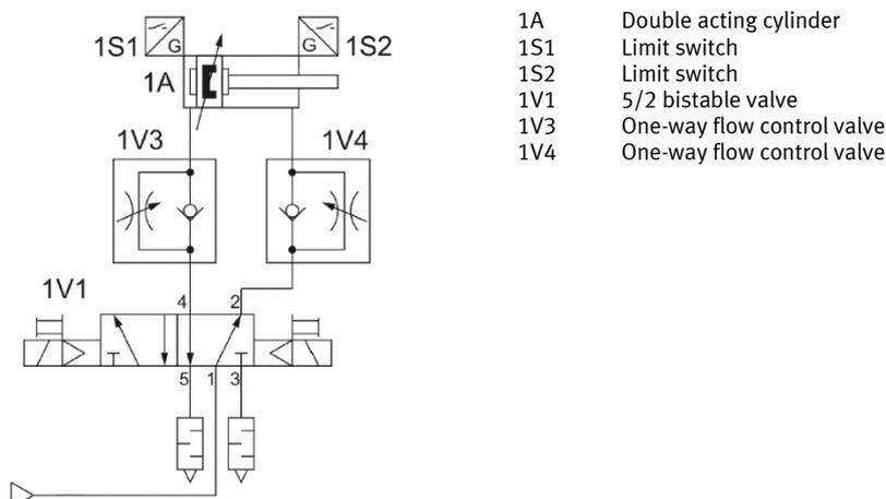
Figure 1: Standard circuit for a double-acting cylinder
