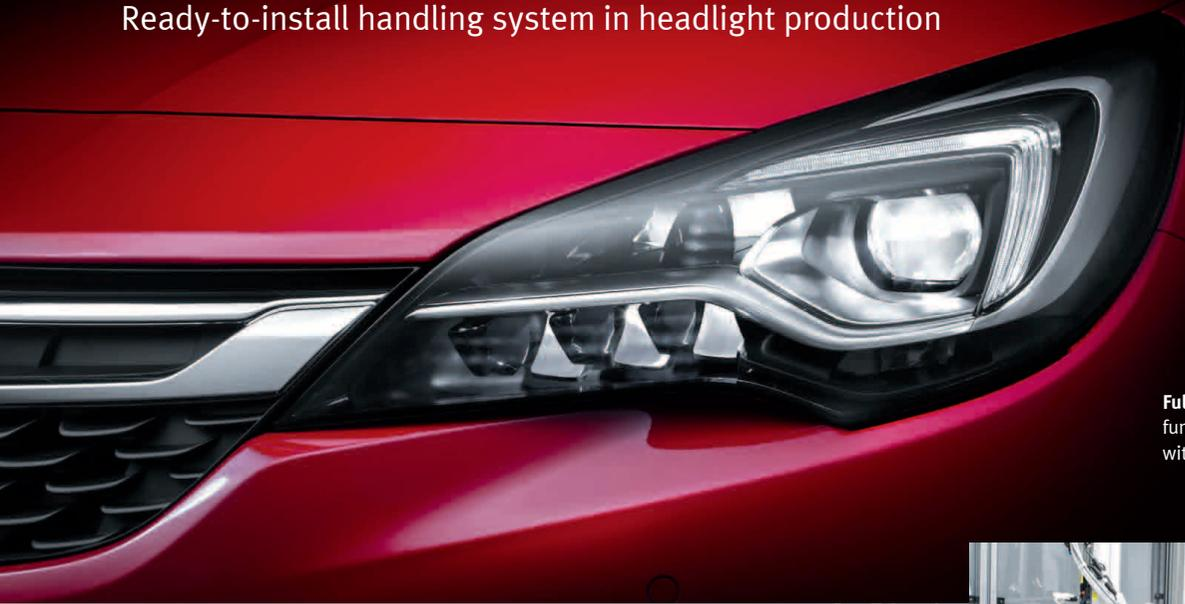
**Full LED headlight** with matrix function for optimum light output without dazzling.
