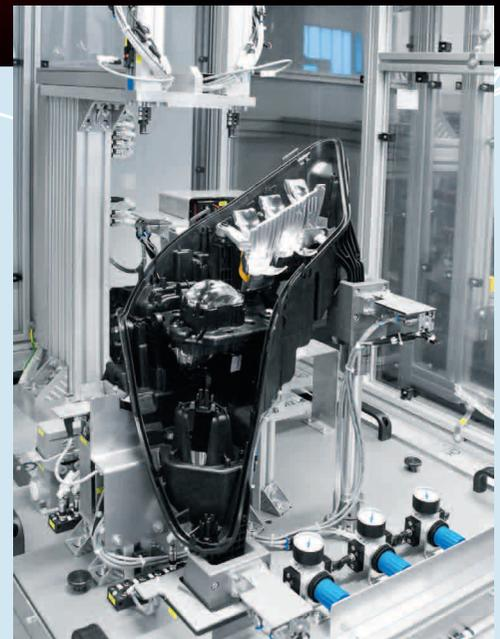
**DSL swivel/linear drive units** pull on the light module and check that it is firmly positioned.
