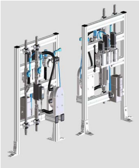
Standard: compressed air and cooling water on different sides
