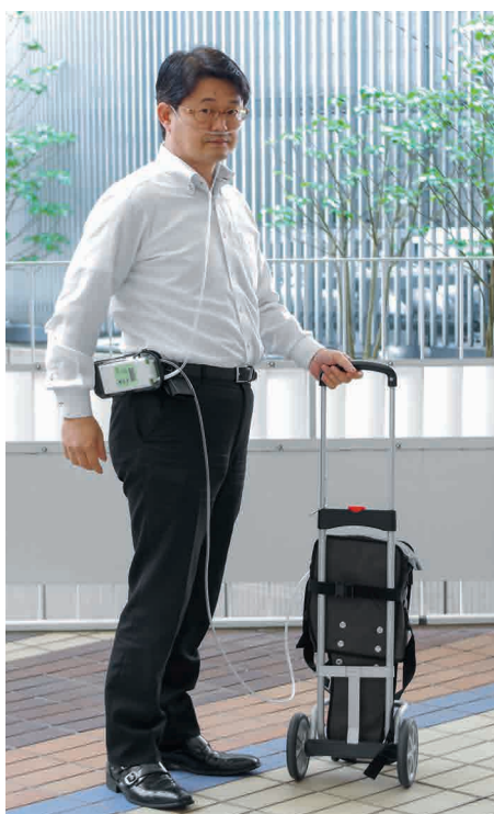
Handy and quiet: the flow regulator IVY can be easily carried and fixed directly on the body.
