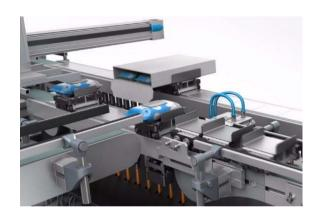
The products to be packaged are transported flexibly to the side loader via the MCS®.
