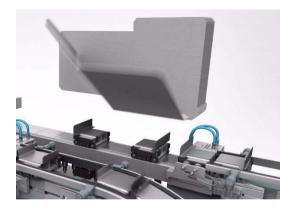
Two carriers hold the box to be loaded. Thanks to the freely positionable carriers, different formats can be transported without any problems.
