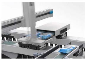
A handling system fills the boxes. The unit consists primarily of an electric axis with motor and a pneumatic mini slide for the Z-stroke.
