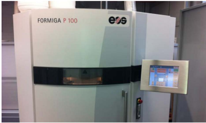
Fig. 3 SLS-Machine for Additive Manufacturing (AM)
