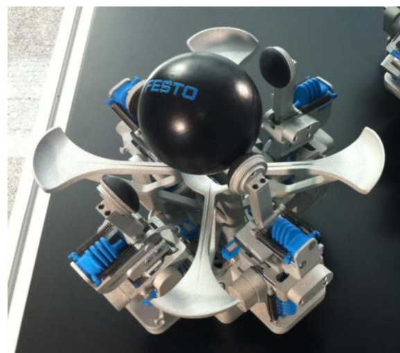
Fig. 13 Final hardware B4-F7 holding a handling object with two fingers
