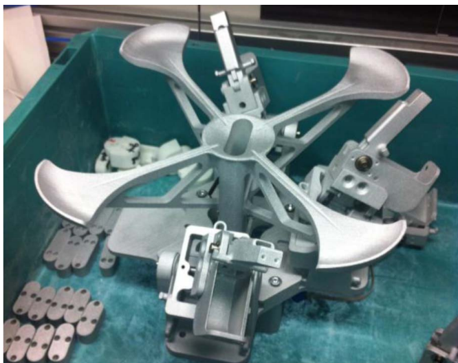
Fig. 10 SLS-generated fallback-frame and a partly-assembled final hand B4-F7
