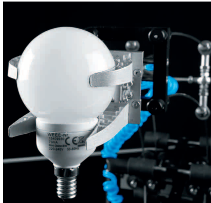
Adaptive gripper: form-fitting and gentle gripping thanks to the structure with Fin Ray Effect®
