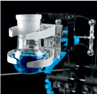
Adaptive gripper: form-fitting and gentle gripping thanks to the structure with Fin Ray Effect®
