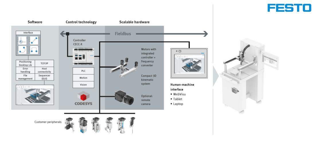
Compact handling system – System structure
