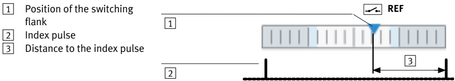
Fig. 2.3 Alignment of the reference switch during index evaluation
