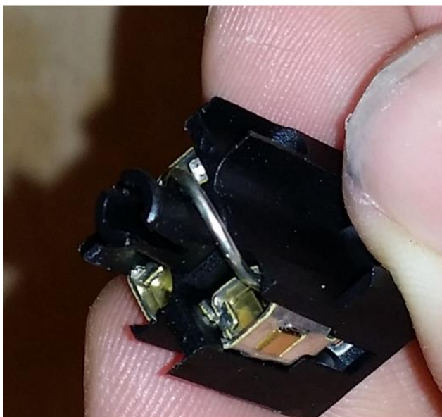
Figure 8: PDAD default status – jumper between terminals 1 and 2 in the insert of the DIN plug
