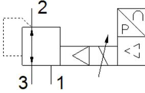
MPPES-3-1/8 is directly control piston regulator. The valve is direct actuated by the solenoid coil.
