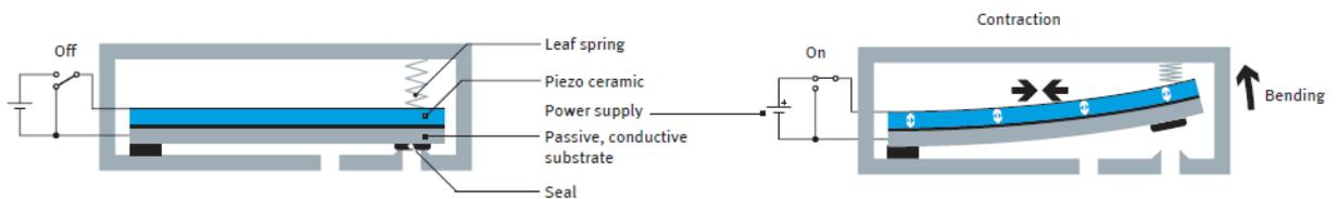
Function of the bender actuator in the piezo valve: when a voltage is applied, the piezo element bends due to a reduction in longitudinal direction.
