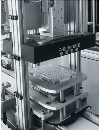
For adding liquid in the microtiter plates in several washing stations, the pipetting head is moved down by an EGSC electric slide.
