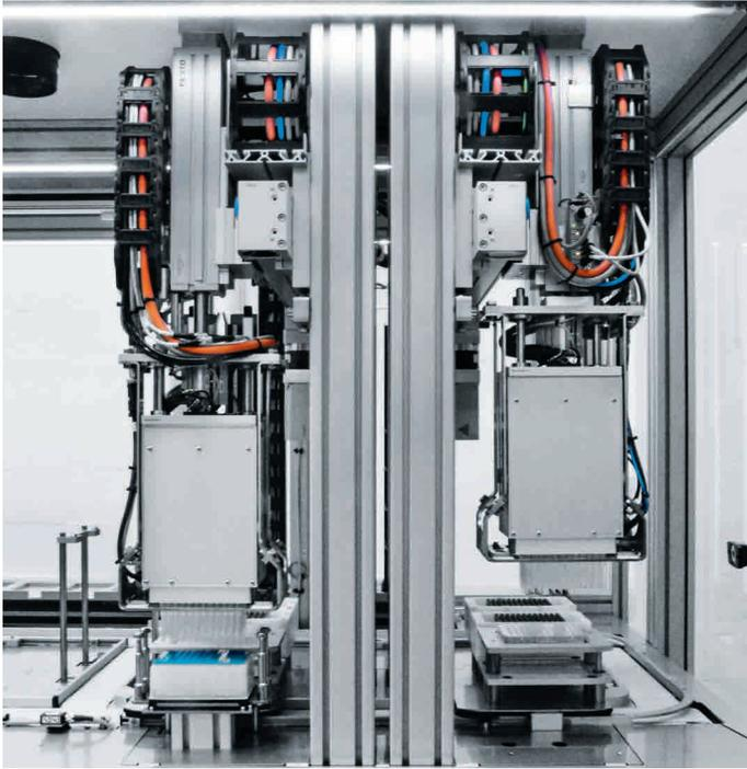
The pipetting head for DNA extraction is positioned by EGC electric axes combined with an EGSL electric slide.
