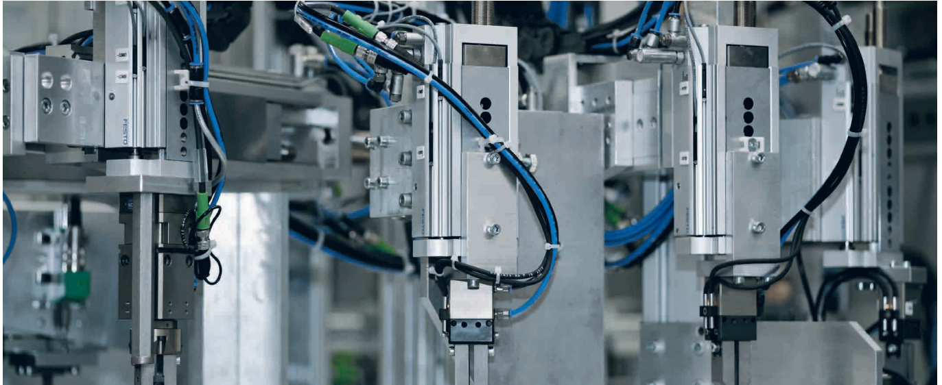
In action: mini slide DGSL as a precise pick & place application in the automotive industry
