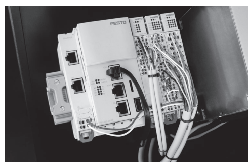
The actuators are controlled by modules on the CPX terminal.
