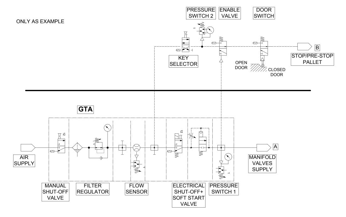
Pressure switch 2 must be supervised by PLC in order to:
