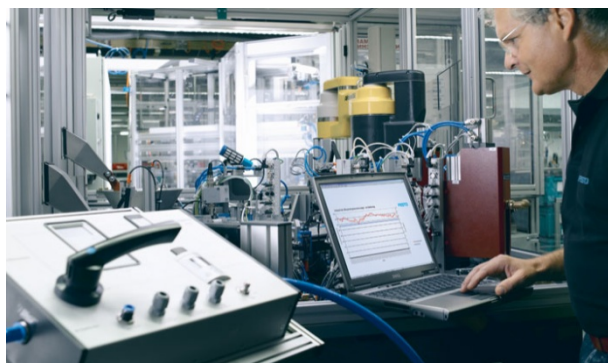
Figure 10: Measurement of compressed air consumption
