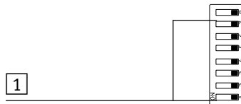
Fig. 1/5: DIL switch 3 (station number)
