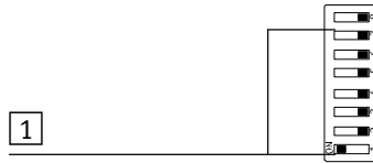
Fig. 1/4: DIL switch 3: (station number)
