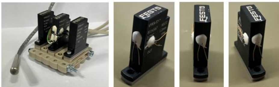
Figure 6: Temperature sensors on VYKA valve
