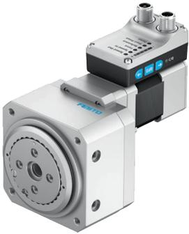
As a cost-effective solution package, the rotary drive ERMS is ideal for simple swivel tasks as well as for increased mechanical loads. The rotary plate has sturdy, precise and backlash-free ball bearings so it can absorb lateral loads and torques.
