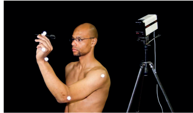
Experimental setup for dart throwing. Markers are applied to the shoulder, elbow and wrist joints.
