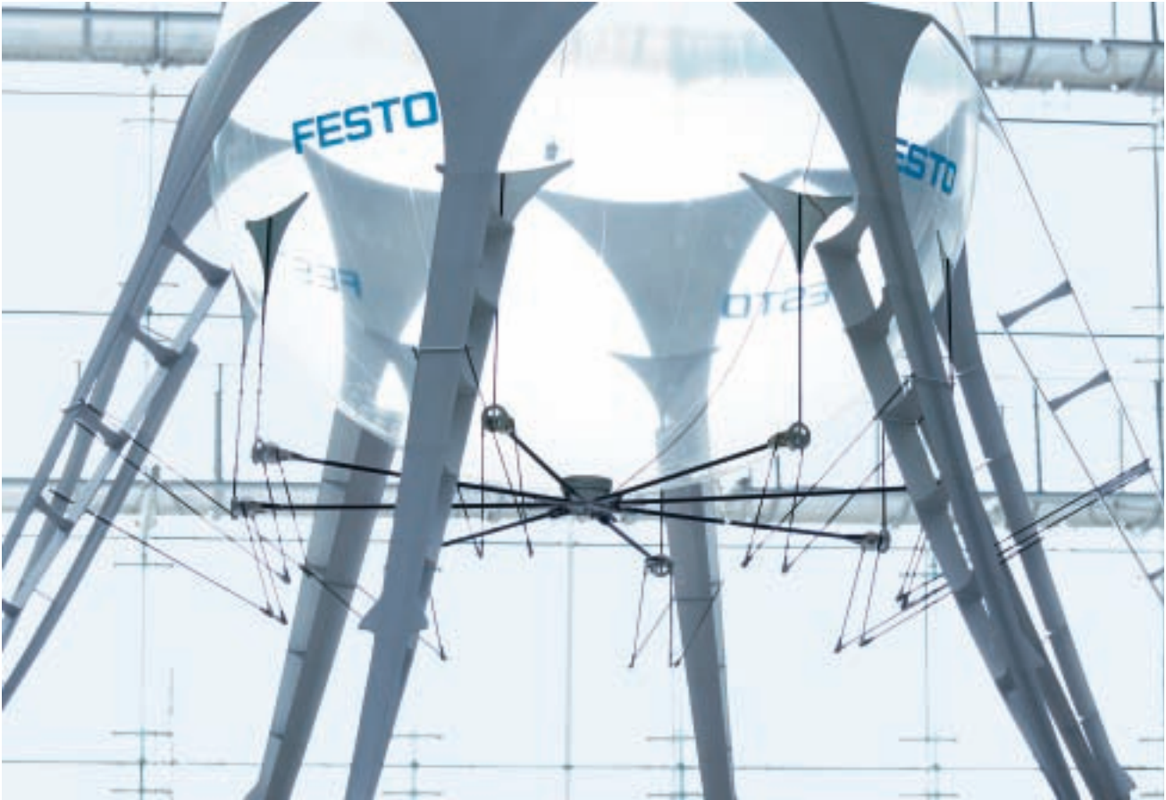
A central electric drive unit with crank mechanism
