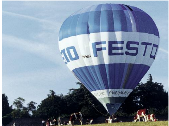
Lift of a hot-air balloon – approx. 275 g/m 3 .
