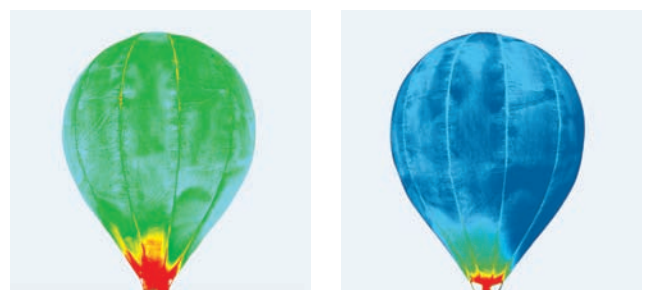
Thermographic images without insulation (left, approx. 55° C) and with insulation (right, approx. 40° C) of model balloons with 30 m 3 volume and identical load-bearing capacity
