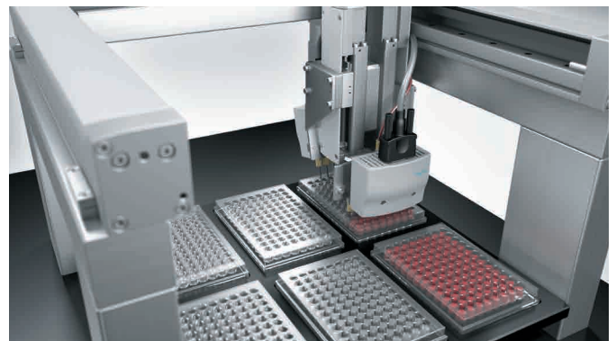
Analysis: controlled aspiration of liquids and precise dispensing in microwell plates.
