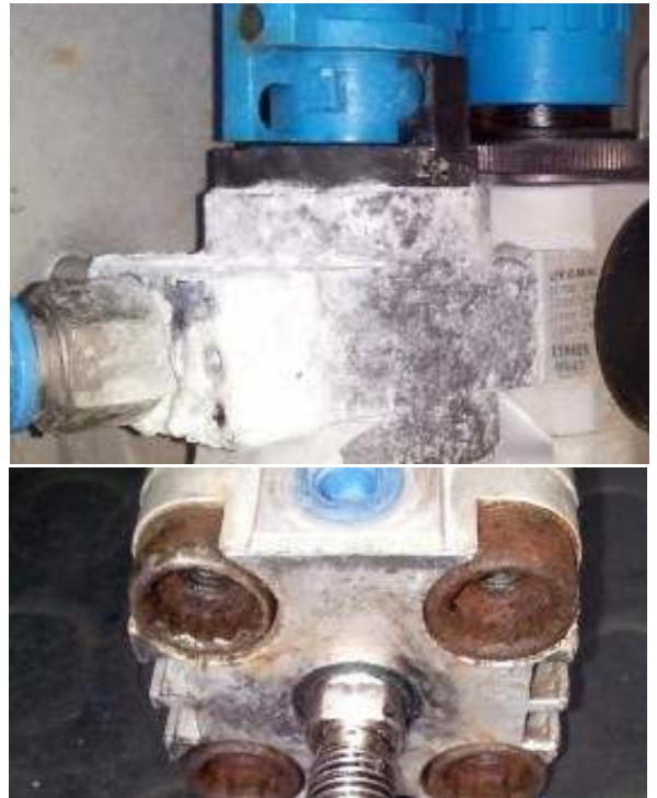
Incorrect choice of materials – typical damage profiles
