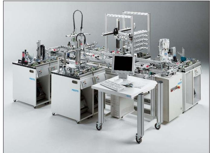
**Adding a conveyor to existing MPS stations enables training in flexible manufacturing:**
