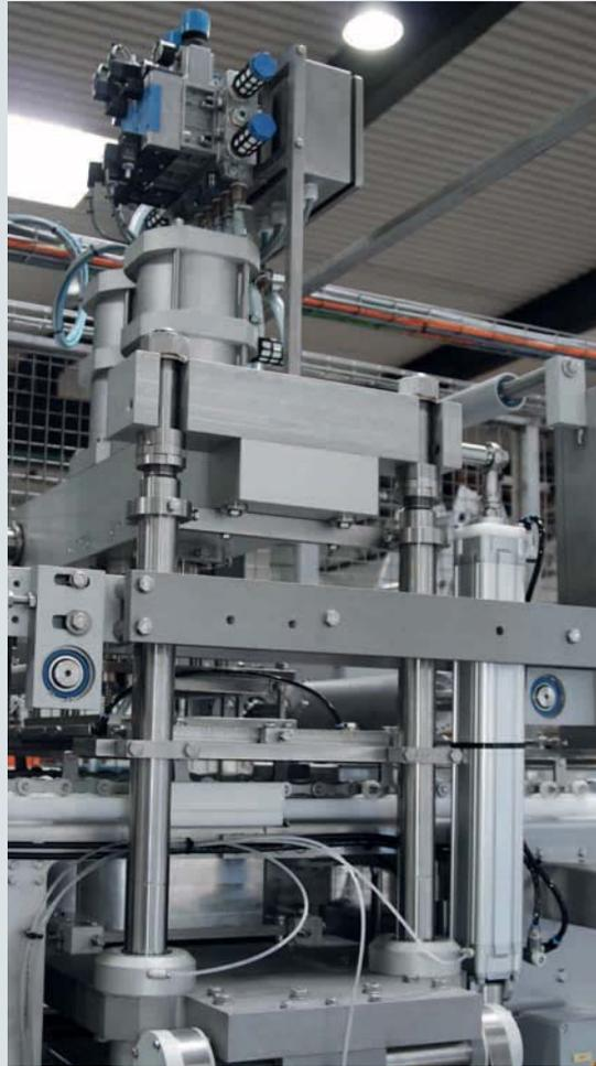
**Output rates** of up to 800 fillings a minute: the RCF robotic filling machine of the “Lieder” brand made by Robot Food Tech. This machine is distinguished by its short set-up times (left).
