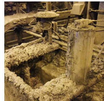
Fig. 6: Pneumatic actuators in flotation cells must withstand harsh external influences. AI helps to identify potential problems early on.
