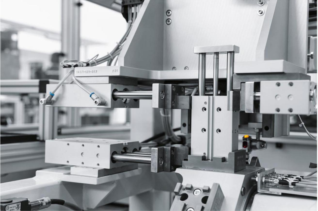
Pneumatic guided drives and slides are the work horses of industrial automation. They are a well-proven concept, adaptable to a growing range of applications where the particular benefits of adding guidance result in superior performance. They are a cost-effective choice as well, with many variants and configuration options to assure great reliability and longevity.
