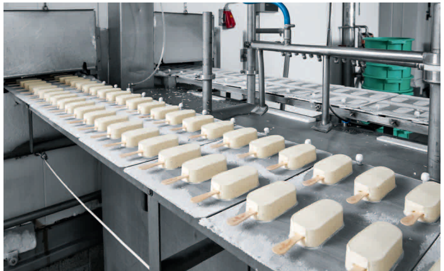
On the belt: one of the five Magnum lines produces more than 20,000 units per hour.
