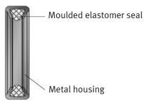
Figure 9: Cartridge seal
