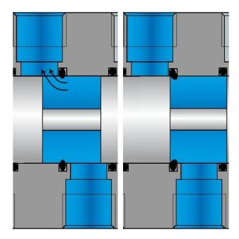
Figure 7: Increase seal wear due to the Bernoulli effect at a pressure of approximately 8 bar or higher.
