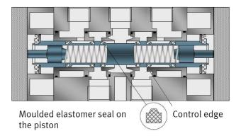
Figure 5: Soft-sealing system with gasket on the piston
