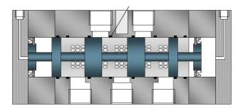
Figure 6: Soft-sealing system with seal in the housing
