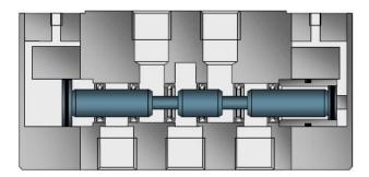
Figure 8: Piston spool valve with cartridge principle
