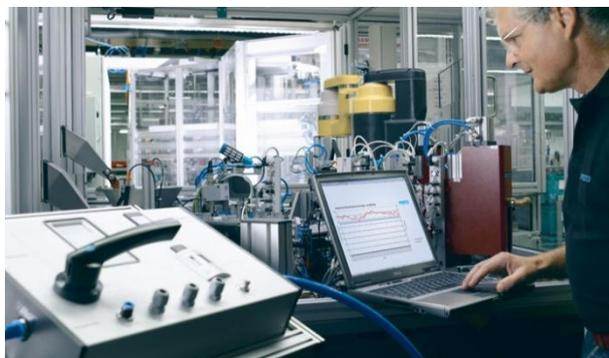
Figure 10: Measurement of compressed air consumption
