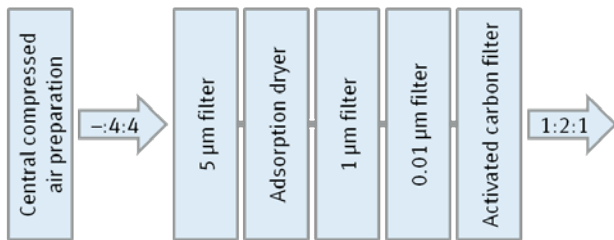
Filter cascade for compliance with class 1:2:1
