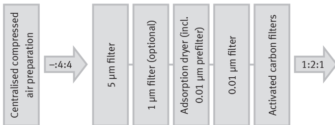
Filter cascade for compliance with class 1:2:1
