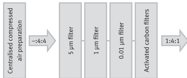
Filter cascade for compliance with class 1:4:1
