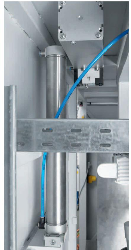
**Landing on the “air cushion”:** Two flange-mounted air chambers ensure that the partition closes quickly yet gently.
