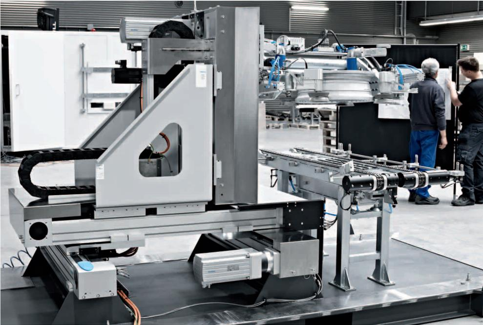
**Ready-to-use precision:** Erhardt + Abt only had to connect the handling gantry with the gripper unit using defined interfaces.
