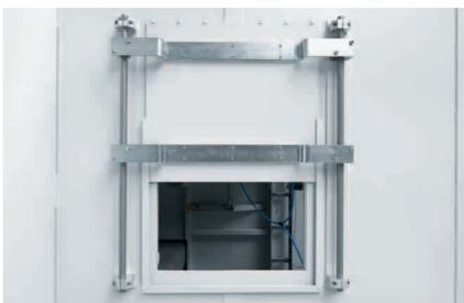
**Lightning-fast trap door:** The 90 kg partition closes in 0.6 seconds and is decelerated at the last moment by a cushioning block.
